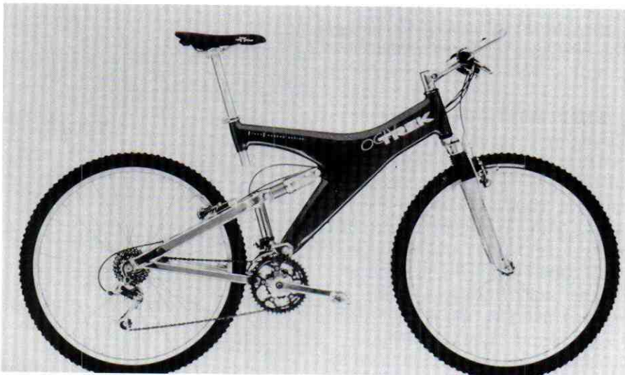
FIGURE 3. This is an adult cross-training mountain bike. It has a shock absorber built into the frame. This bike frame is flexible. It can bend in the area under the seat. Courtesy Trek® Bicycle Corporation.
