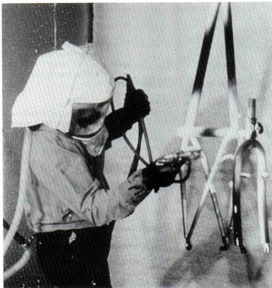
FIGURE 4. Here we have a craft person painting the frame of the bike. The painter will hand spray the tight spots, and then a machine will spray the whole thing. This picture allows you to see the three triangles of the frame. Courtesy Trek® Bicycle Corporation.
